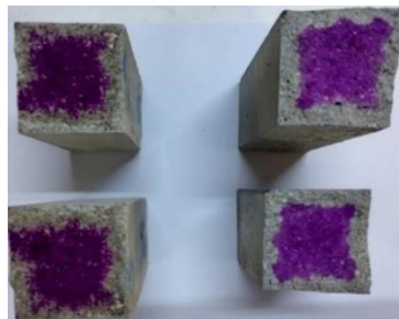
Figure 5-1. Determination of the carbonated layer thickness using phenolphthalein, two years after the initiation of the process
